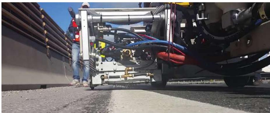
**PINTABANDAS CON DISEÑO MODULAR DE BASTIDOR
