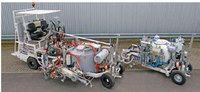
**PINTABANDAS CON DISEÑO MODULAR DE BASTIDOR
